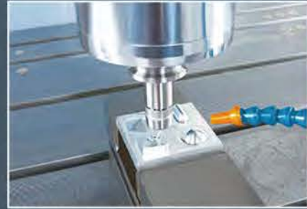
Standard work piece cutting test
