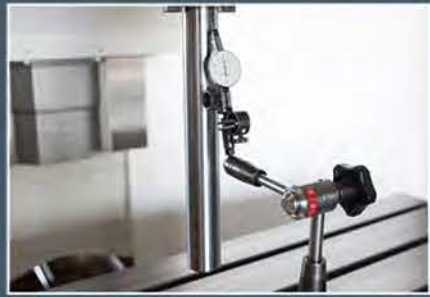
Spindle run out inspection test
